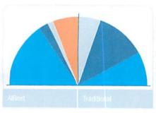
In a compressor installation, a 1 bar pressure drop leads to 7 % more energy consumption. AlRnet offers minimal pressure drop and thus more savings. The leak-resistant and corrosion-free pipes and fittings prevent downtime and ensure high efficiency.
